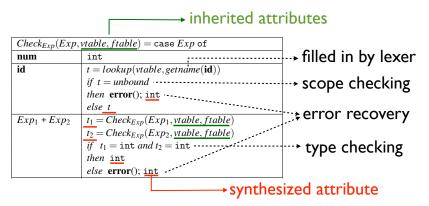
Follows the implementation of slide 249 with one function per nonterminal, with a switch on production rules. Could be implemented with classes/methods or a visitor pattern.
